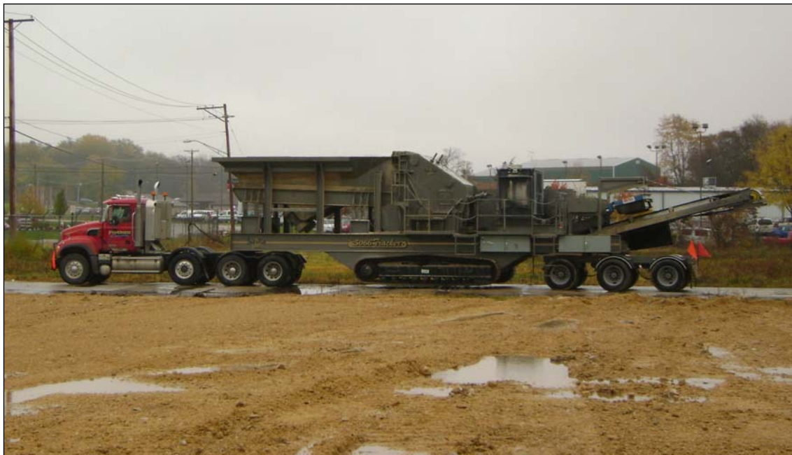
5066 Tracker features quick and easy transport capability using built-in 3 axle bogey and requires no escort.
