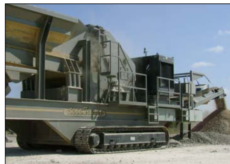
5066 Tracker diesel engine drives crusher, hydraulic pumps for tracks and clutch, and generator for all electric motors.
