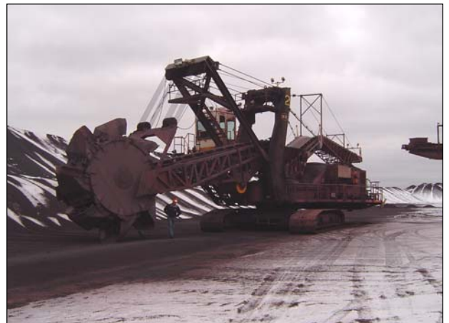
One of three 40 year old bucket wheel reclaimers outfitted with 100 HP Rulmecca Motorized Pulleys. In addition to improving reliability, dual drive system on tail conveyor extended belt life since its 2004 installation.
