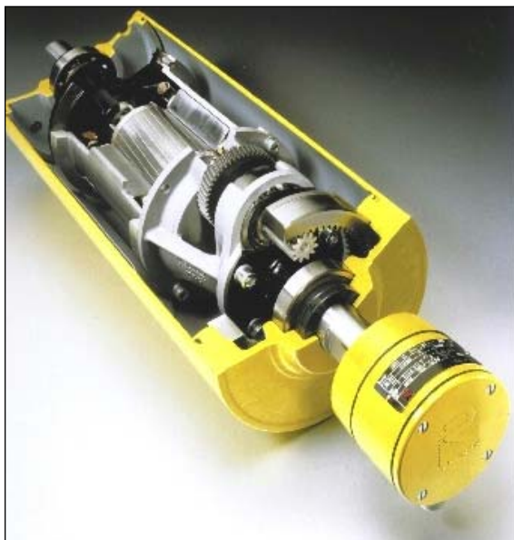
Rulmecca's AC motor and gearbox, hermetically sealed within the oil-filled Motorized Pulley shell, offer high reliability and low maintenance requirements.
